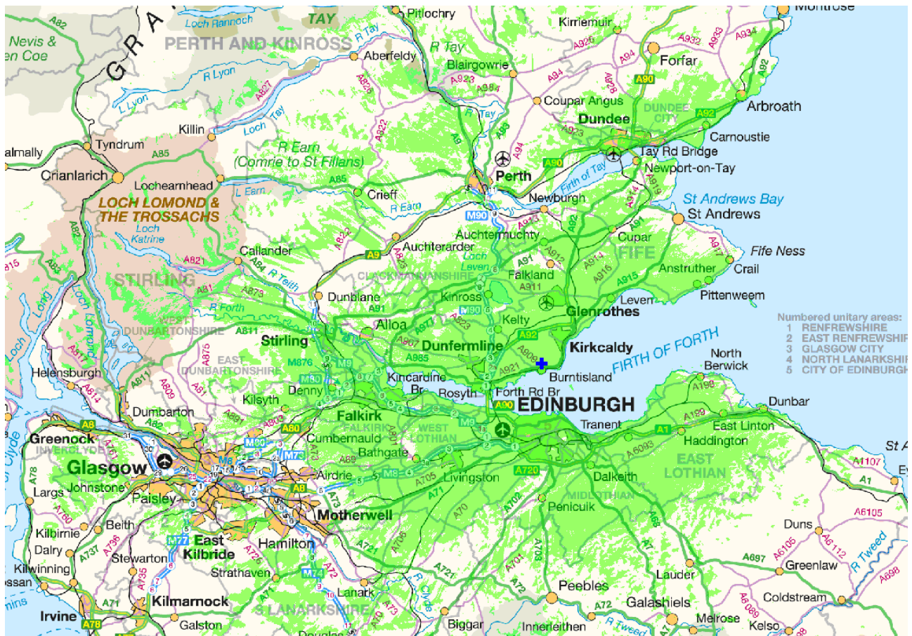
Figure 11: Predicted coverage area for a 1kW DRM+, 4QAM, rate 1/3 station
